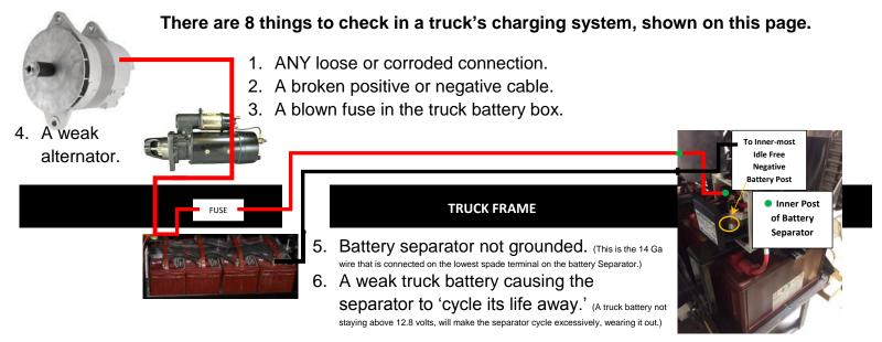
7. A poor truck to idle free ground connection. 8. Cable disconnected after truck battery work.
