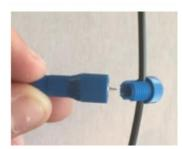
b. Find the correct Start-Stop ignition wire and strip off 3/8" to insert into the connector. Do not twist the wire. Unscrew the smaller end of the Posi-Tap® connector and put the Start-Stop wire through the cap. Allow the stripped wires to surround the Posi-Tap® post. Screw the cap back into the connector. Screw in tightly.
