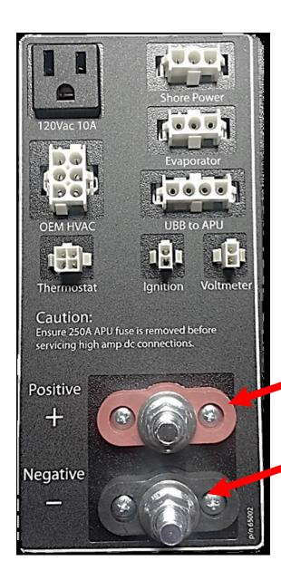
Connect IFS harness 922013 to these connection points on the backside of the UBB.
