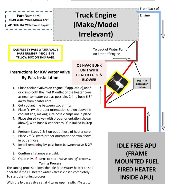
heat, & put AC switch on 'Max AC'. Confirm heater runs for 5 minutes. If it does, that is the end of the tuning process. Due to truck cooling system condition, & as ambient
