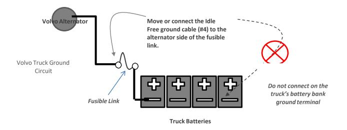
The Volvo Fusible link is located behind the truck's battery bank on the truck's frame.
