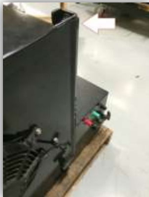
Without Gusset (Defective)
