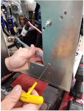
9. Install Mounting plate, and insert flat head bolt into countersunk hole, re-install start capacitor (C-clamp bolt hole facing outside of unit)
