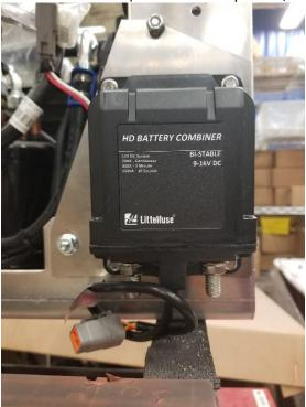
11. Remove cable going to inside of green Marinco (32050) and replace with long cable in kit (32122), install on separator
