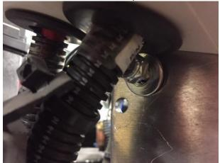
5. Install mounting plate (slot goes under nut you loosened in step 4, bottom left hole should line up with hole that was previously used for battery separator, use bolt from separator to hold bracket in place)
