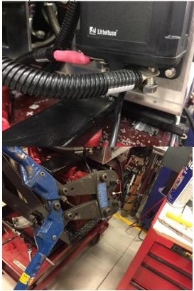
13. Cable coming from Battery (gang cable – 32062 on 3.7 system or Cable - 32039 on 3.6 system), cut off existing lug, strip and crimp on 3/8" lug and install heat shrink
