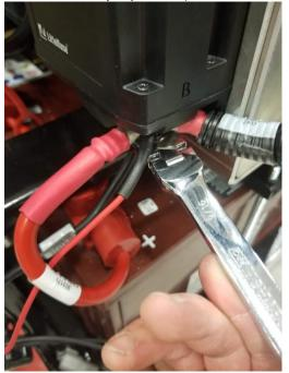
15. Cut off existing ground spade connection on the 32051 cable, strip wire and crimp into new ground wire butt splice, use heat gun to melt Perma-Seal heat shrink, connect Deutsch connectors from ground wire to battery separator
