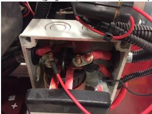
3. Remove battery separator from frame (if 3.7 remove protective box as well)
