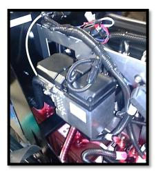
The Webasto TSL17 is a 17,000 BTU coolant heater that is connected to the engine's coolant circuit. When the truck's engine is running, the engine's coolant is circulated through the engine block, cab heater core, Idle Free coolant heater and bunk heater core.
