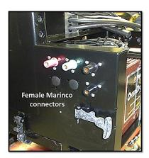
The APU has four Marinco connectors located on the rear side of the frame rail unit. The Marinco connectors are red, green and black, four in total. The male connector is a twist to lock/unlock, connector type.
