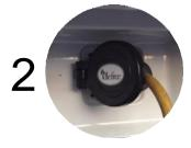
Plug extension cord into the Idle Free shore power receptacle
