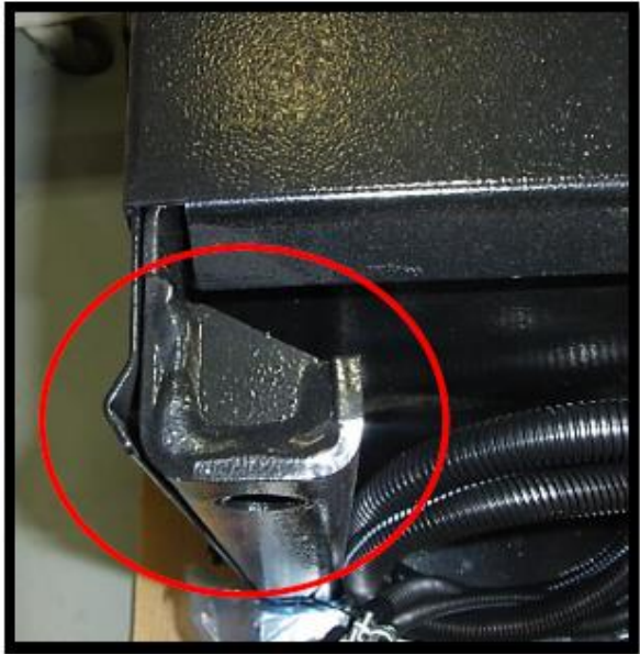
Figure 2 - Frame gusset in place
