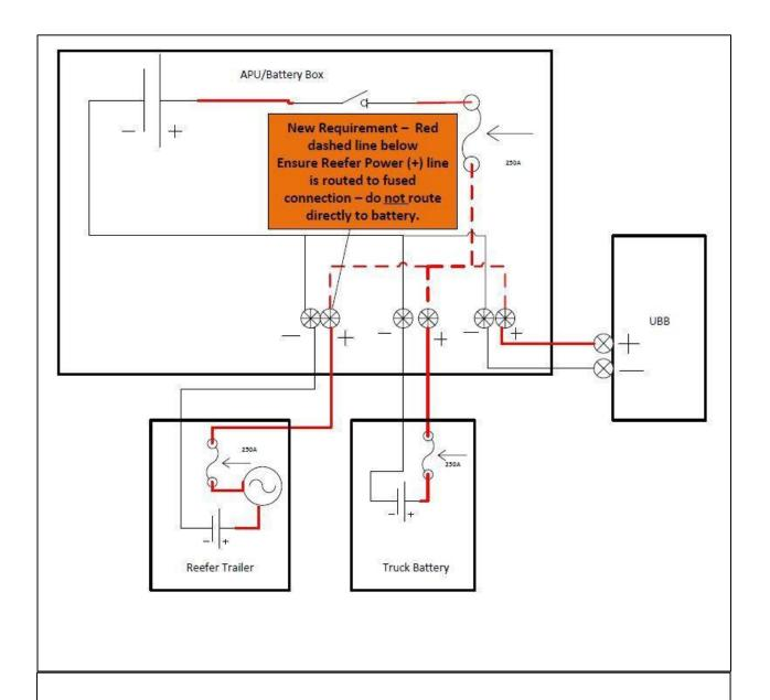
Ensure that the Reefer Link red (+) cable connects to the corresponding red (+) connector and <u>not</u> directly to the APU/Battery Box post. This circuit needs a fused power source as shown in the above schematic.
