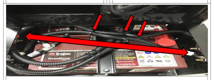
The new red (+) cable should look like the above picture going across the APU battery box connecting to both red (+) connectors. Using cable ties secure the cable. Re-install the battery (-) connections. Apply corrosion preventative to all contacts.
