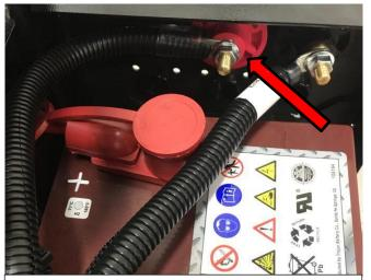
Install the new red (+) cable to its Reefer Link connector shown above. Install second end of new red (+) cable to APU red (+) connector (Left Picture Arrow). Torque flange nuts to 65 in-lbs.
