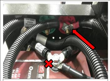
Disconnect the battery (-) connections shown in the above picture with an 'X'.
