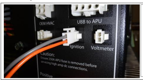
**UBB**: Insert new harness into the Ignition port.
