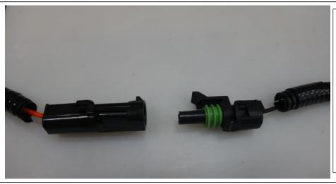
**APU**: Insert new **Orange** wire into the single **Black** wire terminal.
